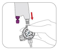
**2** Detach the Air Regulator from the spray gun body by moving it downward.
