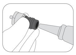
**7** Dry the threads of the nozzle with the Blow Gun AG-6.
