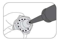
**4** Dry the slits of the nozzle with the Blow Gun AG-6.
