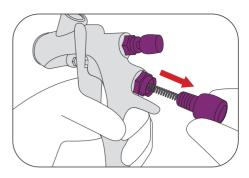
Unscrew the fluid adjustment knob by hand and take it off togheter with the spring.
