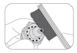
3 Clean the slits of the fluid nozzle using the Brush in Bamboo.
