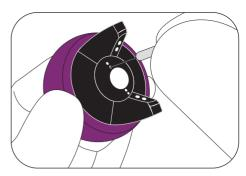
Clean the tiny holes right next to the central hole of the air cap using a proper Cleaning Needle.
