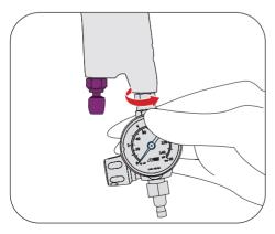
1 Unscrew the Air Regulator connecting nut counterclockwise.
