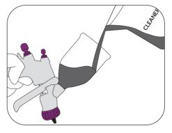
Pour the cleaner into the gravity cup, leave it to act for a few seconds and carry out a preliminary wash to remove any excess of residual paint.
