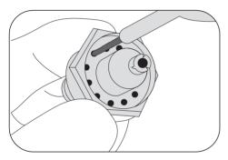
Clean the lateral holes in the nozzle using the Tiny Twisted Brush (ø 3 mm).
