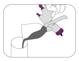
1 Drain remaining paint from the gravity cup into a suitable container and clean the cup with a dry cloth.
