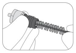
5 Clean the fluid nozzle inside, using the Twisted Brush (ø 10 mm).
