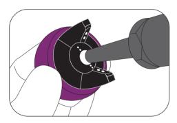
Blow dry the tiny holes right next to the central hole of the air cap.
