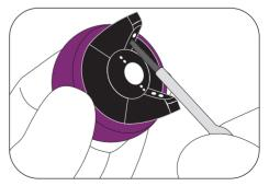
Clean the horn holes with special Tiny Twisted Brush (ø 3 mm)
