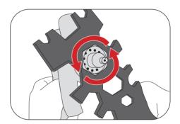
4 Remove the fluid nozzle utilizing the included Spanner.
