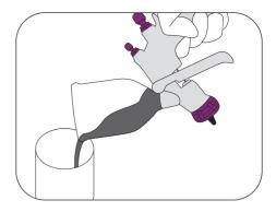
3 Drain the dirty cleaner from the gun and from the gravity cup, into a suitable continer. Repeat the procedure until the cup is perfectly clean and wipe it with dry cloth, then proceed with cleaning of all other parts.
