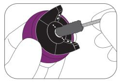
9 Clean the air cap center hole with Twisted Brush (ø 5 mm)
