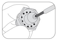
2 Clean the central hole of the nozzle using the Tiny Twisted Brush (ø 3 mm).
