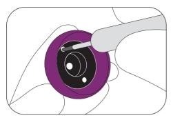
Clean the inner horn holes, and blow dry air cap once finished.
