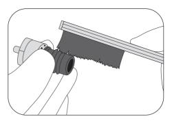
6 Clean the threads of the fluid nozzle using the Brush in Bamboo.
