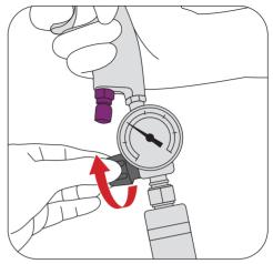
While pulling the trigger, make sure the pressure is set correctly on the external air pressure regulator and corresponding to the technical data sheet.
