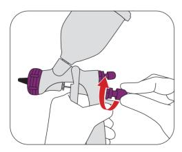
To decrease the fluid delivery, turn the fluid output adjustment knob clockwise.
