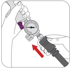
**2** Firmly assemble the gravity cup to the spray gun fluid nipple.
