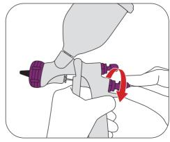
To increase the fluid delivery, turn the fluid output adjustment knob counter-clockwise.
