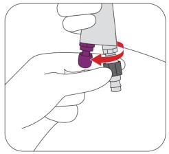
1 Connect Pressure Gauge and/or air nipple to the air inlet port of the gun.
