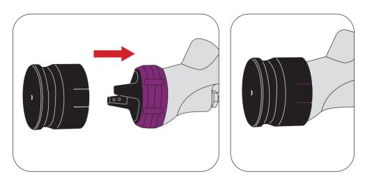
1 Simply put the UV Protective Cap onto the air cap of your WS-Primer spray gun.
