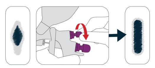
**2** Turn the pattern adjustment knob counter-clockwise
