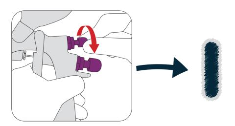
2 Turn the pattern adjustment knob counter-clockwise to achieve a flat & thin fan pattern.
