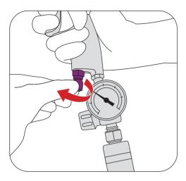
**1** Fully open the air adjustment on the spray gun.
