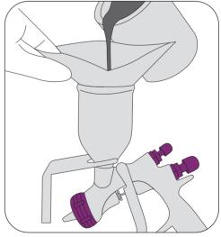
Pour paint into the gravity cup by filtering it by an appropriate strainer to eliminate all impurities.
