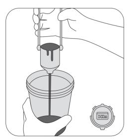
3 Check the correct viscosity of the paint as recommended by the paint manufacturer.
