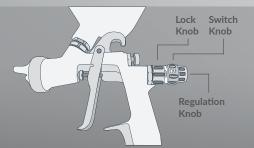
2. The regulation knob is used to adjust the desired paint delivery. The lock knob fixes the position of QFA on the spray gun. The switch knob changes the paint delivery.
