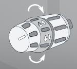
**3.** The switch knob has two positions; rotating counterclockwise provides full paint delivery, while rotating clockwise provides reduced paint delivery.
