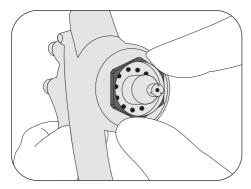
Reassemble the fluid nozzle tightening it 1 manually into its seat.
