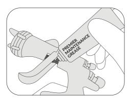
Apply a small amount of grease to the 11 fluid needle in the trigger slide area.
