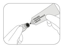
Lubricate the fluid needle ajd. knob with a small amount of maintenance grease.
