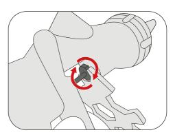
Now attend to the adjustment of the 12 fluid needle packing. Screw the needle packing nut tight by the spanner until the needle starts to stick.
