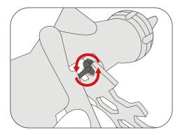
Once the needle sticks, unscrew the needle packing (counter-clockwise) until the needle just moves freely again.
