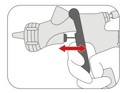
Check the smooth sliding of the fluid needle by pulling the trigger few times.
