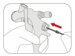
Insert the lubricated fluid needle set carefully into its seat.
