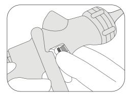
Place the self-adjusting needle packing in 5 its seat and tighten it manually.
