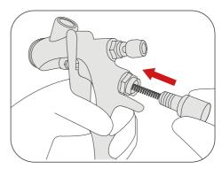
Reassemble in the following order: the 10 needle spring and then the fluid adj. knob set.
