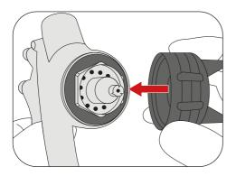
Reassemble the air cap. 3
